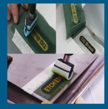
TIG Brush Marking is the best the market has to offer with exceptional results. It just takes 10 seconds to produce a mark with the TIG Brush Marking System. The TIG Brush changes the pigment from silver to black, keeping the passivation layer intact (whereas other systems on the market bring the carbon from the stainless steel to the surface to create the mark). Marking is also adaptable to aluminium, giving a vivid white mark instead of black.
